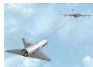
Tow launch of a Kelly Space and Technology Astroliner (Photo: Kelly Space and Technology, Incorporated)
