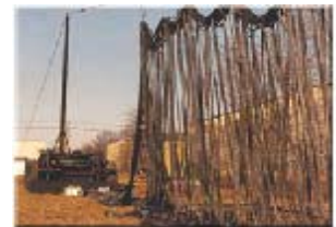
Ground-based arresting gear (Photo: Engineered Arresting Systems Corporation)
