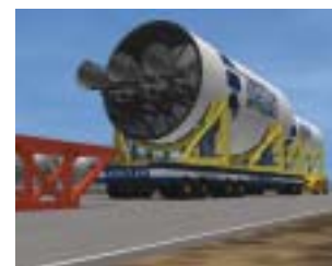
Horizontal transport of the vertically launched Kistler Aerospace K-1 (Photo: Kistler Aerospace Corporation)
